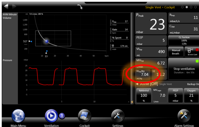
Fig. 3 Ventilation with AVM of a 70kg patient. V_t/kg is 7.04 ml/kg, clearly above the recommended tidal volume for lung restrictive patients.
